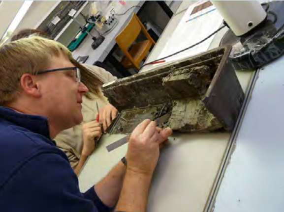
Taking samples according to layers (may be only 2mm thick!)
