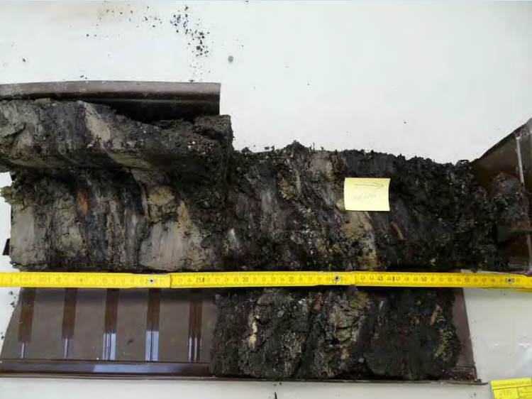
Taking samples according to layers (may be only 2mm thick!)
