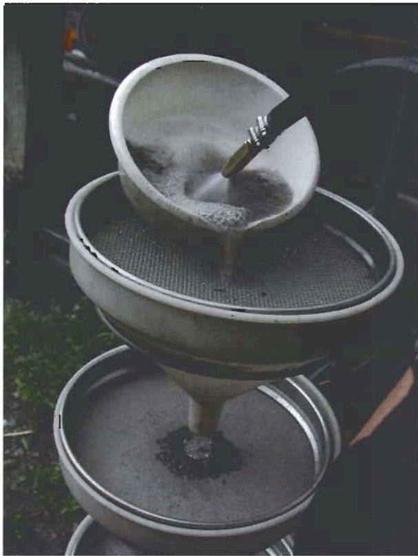
Figure 14 Sieving of a sample, using the wash-over technique. Photograph by D. Hager, © IPNA, Basel University.
