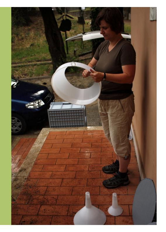
A "window" is cut into the two wide stackable boxes which already contain a hole for the funnel and sieve so that the content of the sieves can be controlled at all times.
