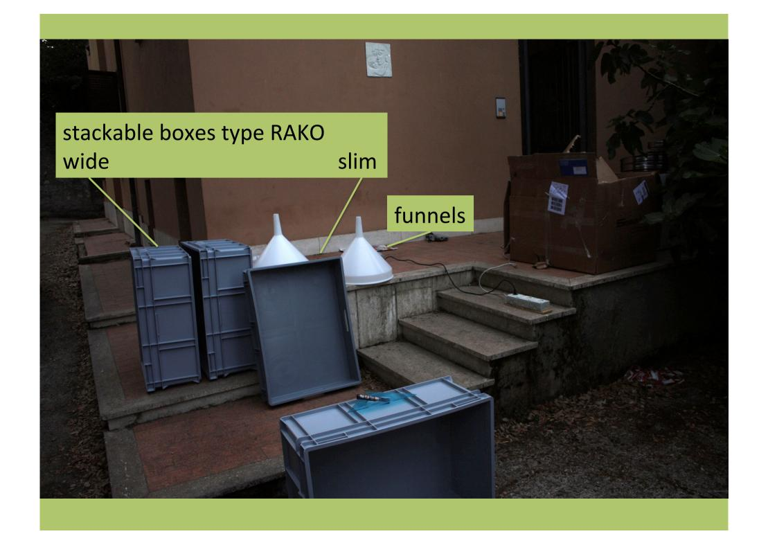
A hole for the funnel (Ø450mm or any other size matching the funnels and sieves) is cut into two of the wide stackable boxes and the slim stackable box
